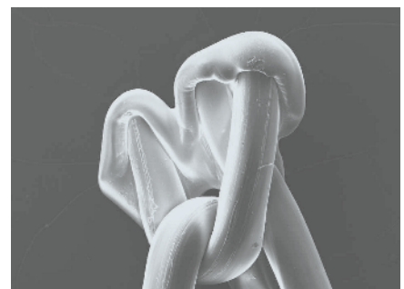
Laser cut for round suture ends
